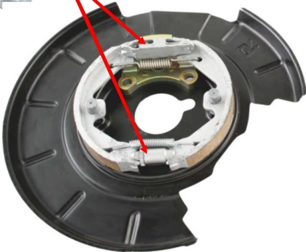
When changing the Brake Shoes, for technical and safety reasons, it is recommended also to change the Accessory Kit, the Brake Adjuster Kit or the Expander Lock Kit. This to ensure even braking ability and functionality.
