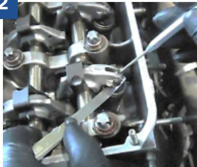
*Adjust the eccentric washer with the valve head by introducing between them a calibrated gauge of **0.25 mm**.*
