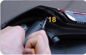
18. With a suitable tool, loosen safety clip from drive's ball pivot seat at the tailgate and remove
