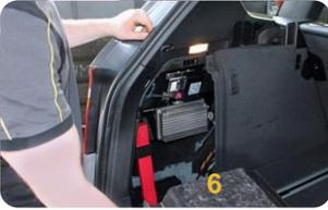
7. To uninstall trunk liner, first loosen trunk liner fastening (2 screws and 3 clips), as well as the trim for the rear seat catches
