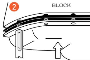
2. Slide oil pan gasket and oil pan into place over the Payen Snap-ups
