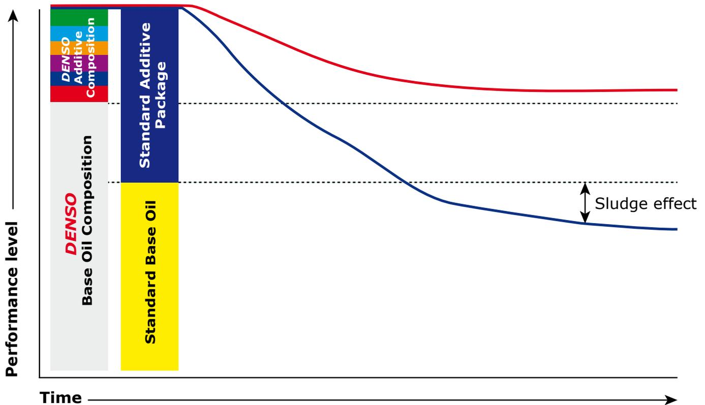
Typical chart of the interaction between loss in performance and additive consumption. Comparison of DENSO ND-oils vs (Ordinary) PAG oils.
