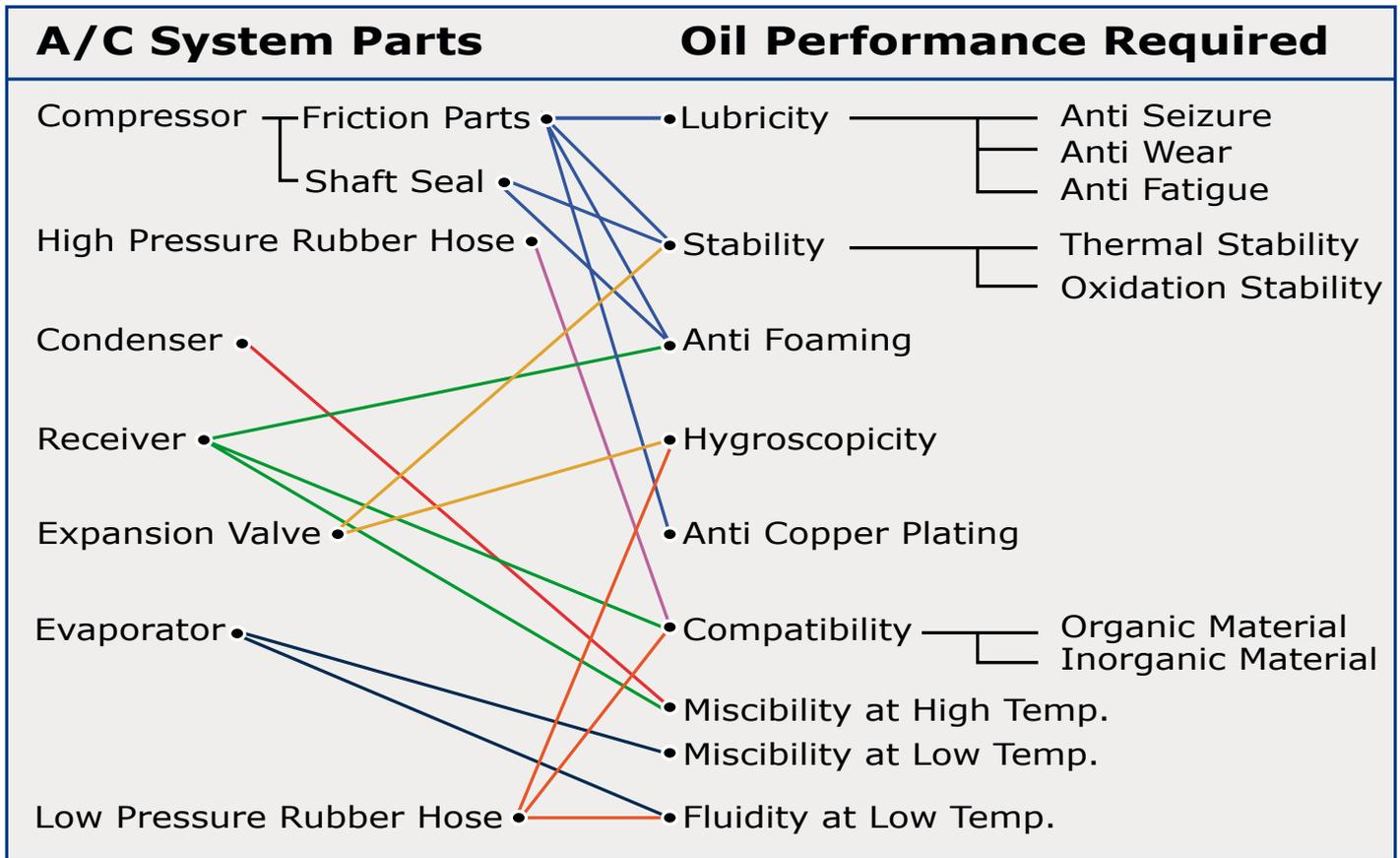
**Examples:** For the expansion valve, Thermal- & Oxidation Stability are important as the refrigerant temperature decreases rapidly after the expansion valve. Hygroscopicity is another important factor at the expansion valve. For compressor inner parts, Lubricity, Stability, Anti Foaming and Anti Copper Plating are important factors.
