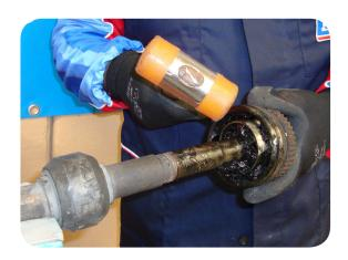
4. Hold the CV-Joint and pull it off the shaft by tapping with a hammer.
