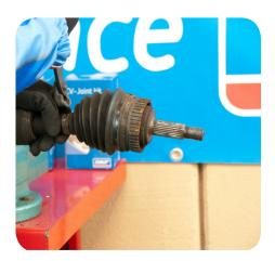
2. Place the driveshaft in a vice (with aluminum or protective jaws).
