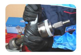
3. Slide the boot into position ready for mounting and fill with all of the supplied grease.
