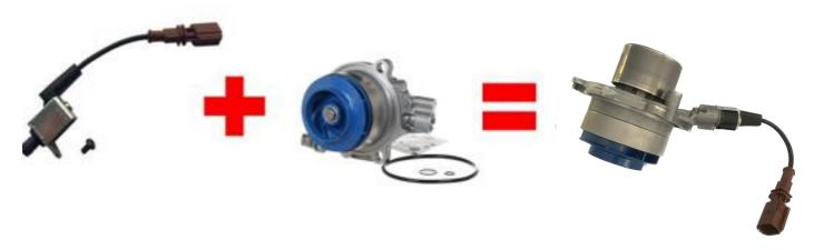
**NOTE**: If the actuator is not fitted correctly, defect code and warning light may appear on the car dashboard!
